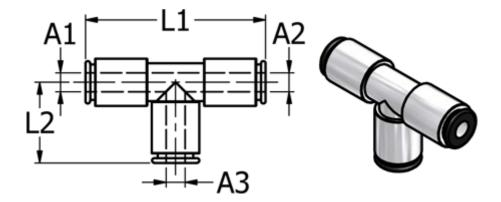
Ext. hose diameter A1 = 5Ext. hose diameter A2 = 5Ext. hose diameter A3 = 5
